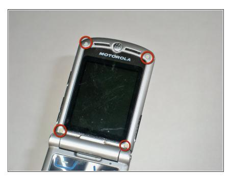
Remove the four rubber pieces from all corners of the area around the screen.
