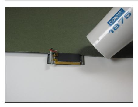
Use the hairdryer to heat each side of the battery for at least 30 seconds.
