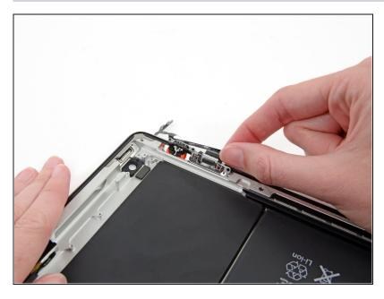
Lift and remove the power & volume button cable out of the iPad.
