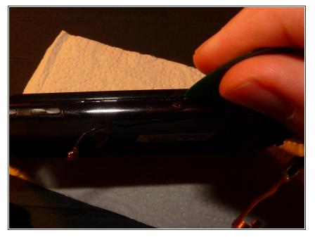
Use the guitar pick to detach the glass housing from the housing of the LCD screen. Be careful, you have to detach a lot of pins. Have a close look at the picture before you proceed.
