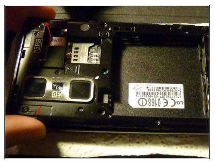
• Loosen up the frame. Remove it carefully with your hand.
