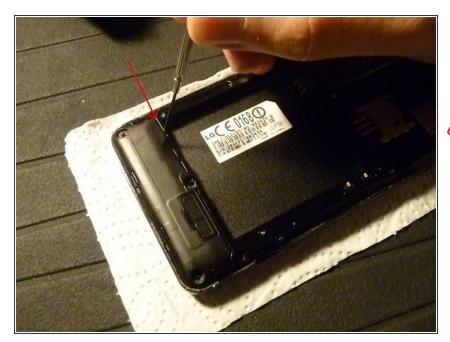
• With the tiny screwdriver go under the bottom plate. Lift the plate and remove it.
