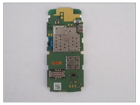
• Place the circuit board with the display facing downward.
