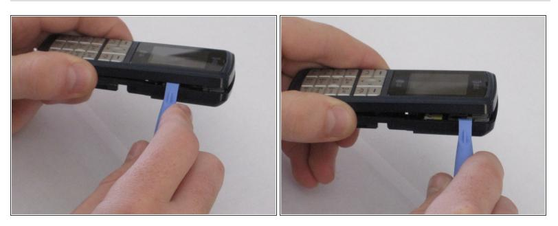
• Run the tool along the seam to release all the tabs.
