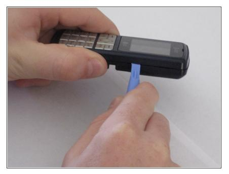
Insert a plastic opening tool in the seam.
