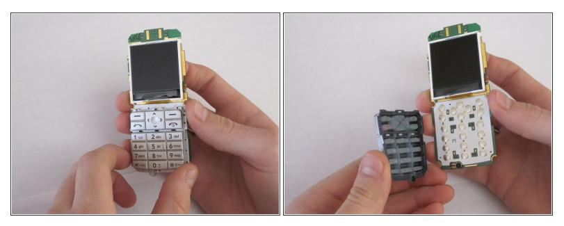
• Separate keypad from circuit board by turning it upside down and allowing it to fall off.
