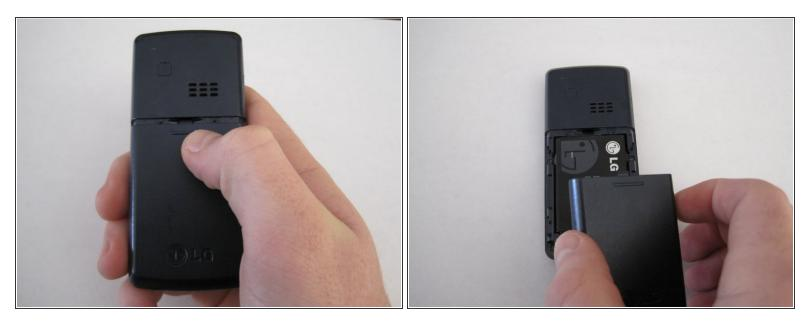
• Slide the back cover down using your finger to remove the cover from the phone.
