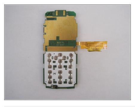
• The circuit board is separated from the rest of the phone.
