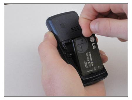
• Press downward while pulling outward to remove the battery.
