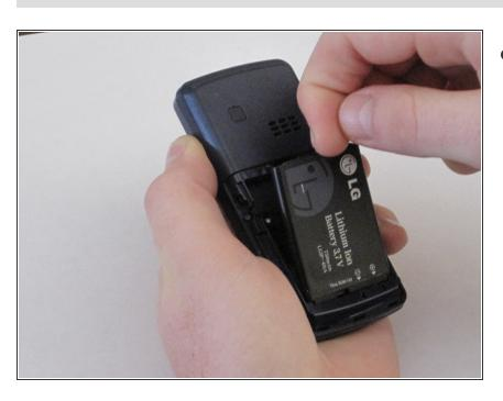
Press downward while pulling outward to remove the battery.
