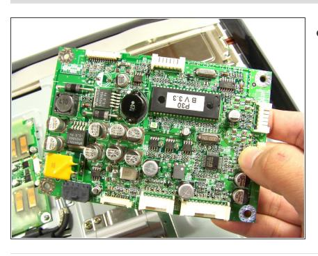
Remove and replace the logic board.
