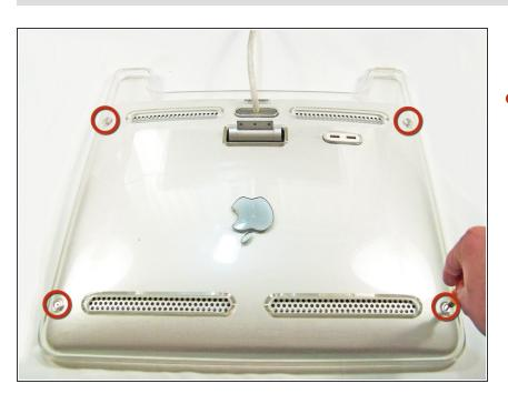
Remove the size 2.5 hex screws from each corner that connects the panels to the display and remove them.
