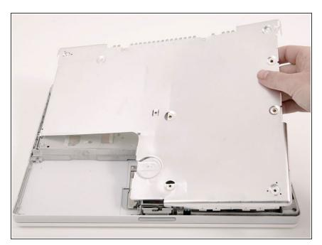
Lift the bottom shield off.
