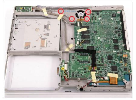
Remove the 4 Phillips screws securing the fan to the metal framework.
