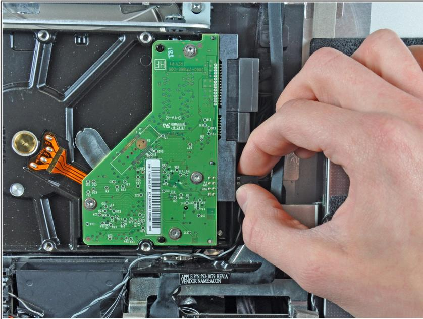
**⚠** Before disconnecting the thermal sensor cable, take note of its orientation. It is extremely important to reinstall the connector **reversed** from the current orientation so the fans will not run at full speed.
