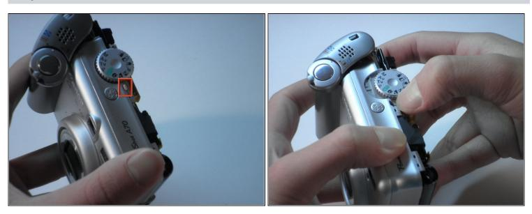
• With your right thumb, pull back on the tab while using your left hand to pull the face of the camera away from the body.
