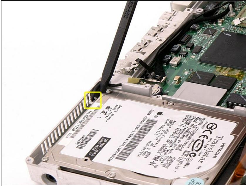
**⚠** The cable you're about to remove is very fragile - do not pull directly on the wires. Instead, try to pry up the connector directly, using a spudger or a small flathead screwdriver if necessary.
