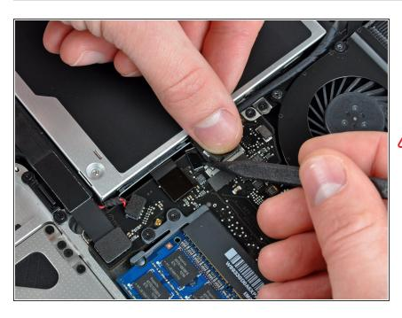
Apple sticks a small strip of clear plastic with adhesive applied to one side to the logic board behind the camera cable connector to keep it in its socket. When moving it out of the way, be sure not to break any surface-mount components off the logic board.
