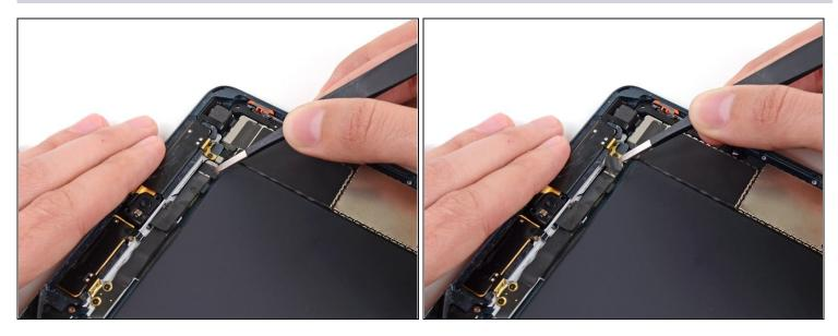
• Use a pair of tweezers to peel up and remove the small piece of tape covering the frontfacing camera cable connector.
