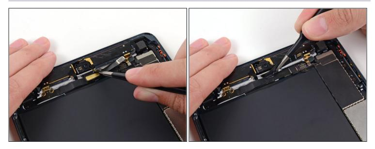
• Gently fold the front-facing camera cable upwards (roughly at a 90-degree angle), exposing the bottom side of it.
