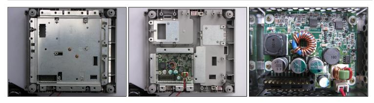
• If you lift the mainboard up, you'll see a metal plate, probably for EMI-protection. Remove the two screws holding it and you have access to the internal power supply.
