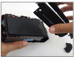
• Loosen the back cover from both the left and the right sides of the camera. Take off the back cover.
