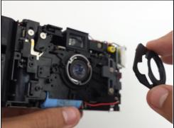
$\triangle$  The lens is only attached to the main camera body. Set the front and back covers aside.
