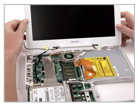
Tilt the display back, freeing it from the two metal alignment posts holding the hinges in place, and slide it away from you.
