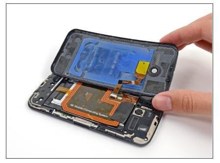
Gently set the back cover down in a way that exposes the camera flash cable connector, but does not put strain on it.
