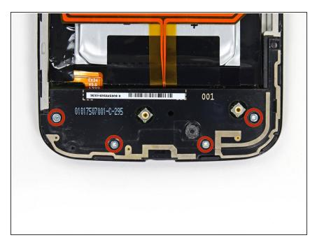
Remove the four 3 mm T3 Torx screws securing the lower antenna assembly to the phone.
