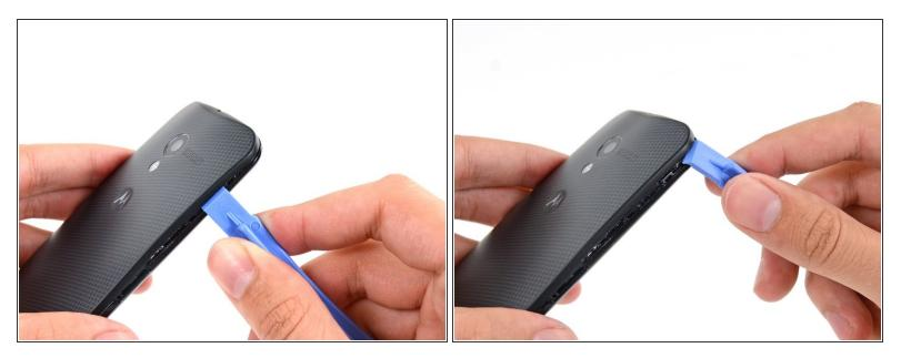
• Carefully slide the plastic opening tool around the corner, freeing it from clips.
