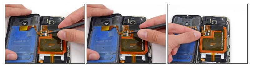
• Use the tip of a spudger to flip up the retaining flap on the flash cable ZIF connector.
