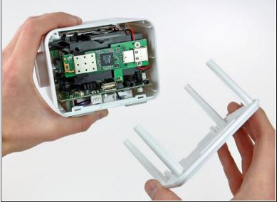
Remove the rear cover from the device.
