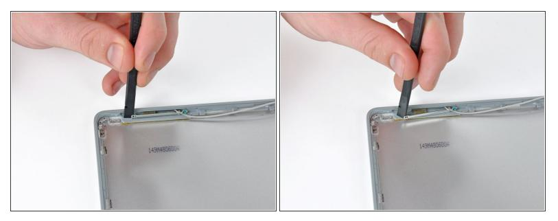
• The antenna is attached to the rear display bezel via adhesive. To remove it, place the flat end of a spudger behind the top edge of the antenna, and carefully twist the spudger to pop the antenna off.
