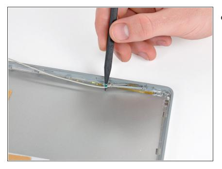
Remove the left antenna in the same way the right antenna is removed (shown above).
