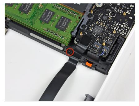
Remove the 3.1 mm Phillips screw securing the hard drive cable to the upper case.
