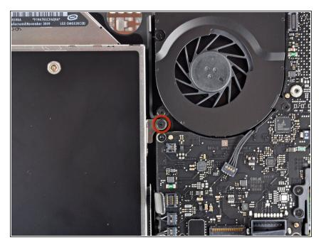
Remove the single 4.5 mm Phillips screw securing the optical drive bracket to the upper case near the fan.
