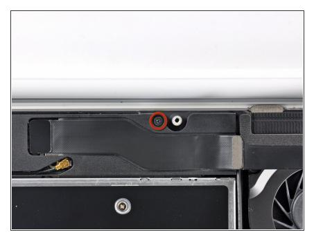
Remove the single 12 mm Phillips screw securing the top of the rear speaker housing to the upper case.
