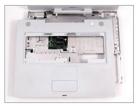
Carefully lift the upper case about half of an inch and move it so that you can access the power and speaker cables.
