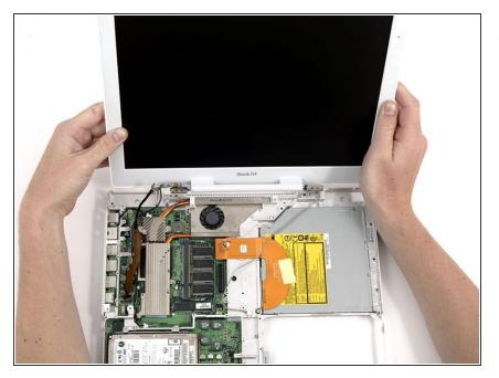
Lift the display up and tilt it backwards, freeing it from the two metal alignment posts holding the hinges in place, and slide it away from you.
