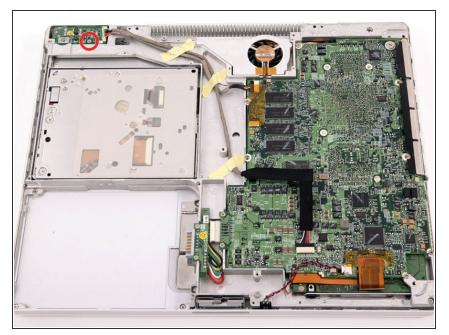
• Remove the single Phillips screw securing the DC-In board.
