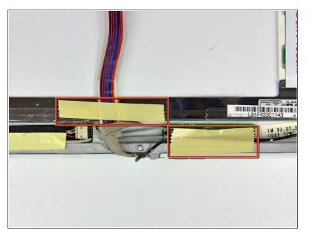
Remove the pieces of tape covering the display data and microphone cables near the bottom edge of the display.
