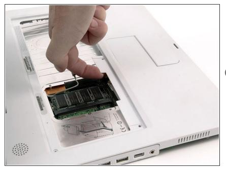
Before you can yank the upper case off, you must disconnect the trackpad connector, the blue and white power cable, and speaker cable as described in the next steps.
