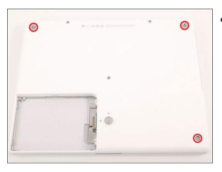
Remove the three newly-revealed Phillips screws.
