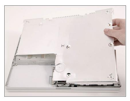
• Lift the bottom shield off.
