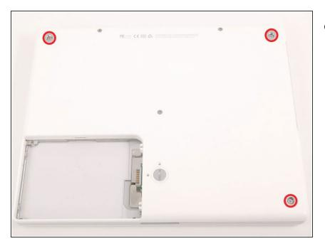
Remove the three newly-revealed Phillips screws.
