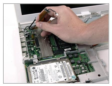
Deroute the microphone and display data cables from the metal framework, removing tape as necessary.
