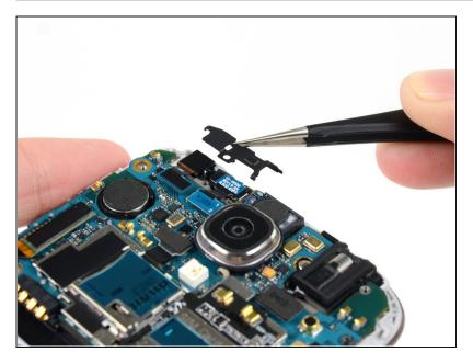
Remove the upper display assembly bracket.
