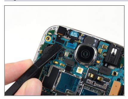
Using the flat end of a spudger, disconnect the front-facing camera cable connector.
