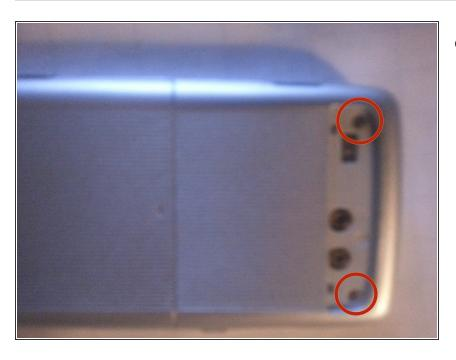
Unscrew the two .4 cm Phillips head screws from under the Samsung logo
