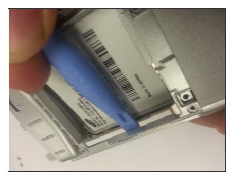
Using the plastic opening tool gently insert it into the seam and work it around till the cover comes off.
