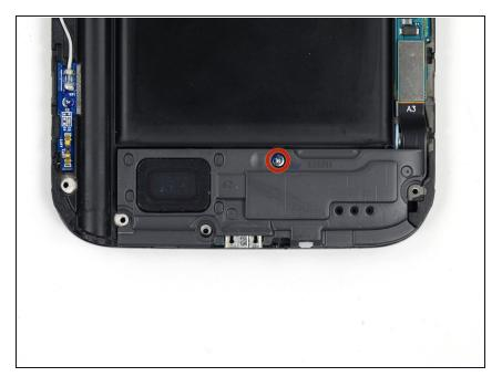
Remove the 3 mm Phillips #00 screw from the speaker enclosure.
