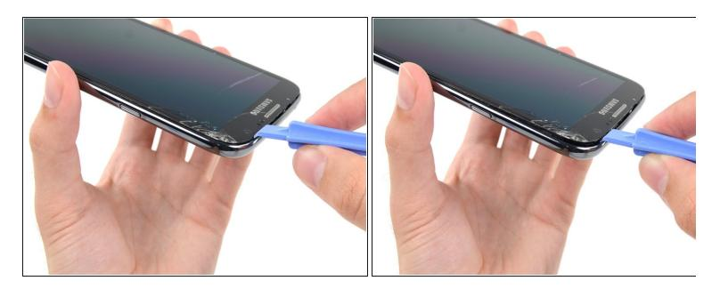
Push the plastic opening tool down to free the corner of the midframe from the display assembly.
