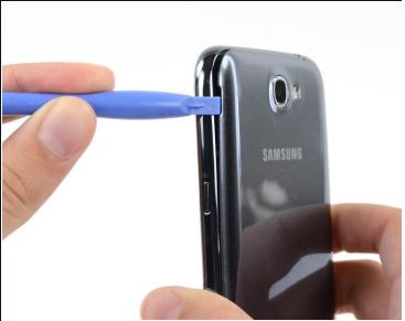
• Pry with a plastic opening tool, or your fingernail, in the divot to the left of the rear-facing camera, near the power button.
