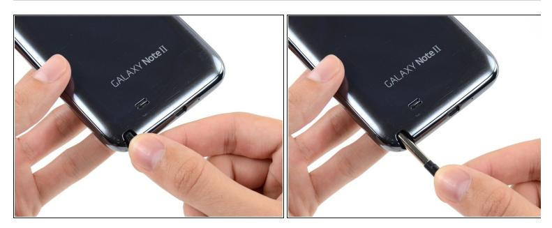
Grasp the end of the stylus and remove it from its slot in the midframe.
