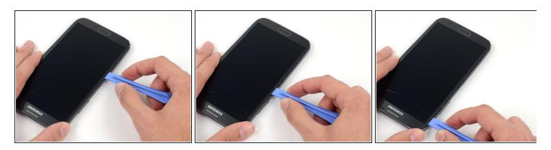
• Continue to run the plastic opening tool down the seam.
