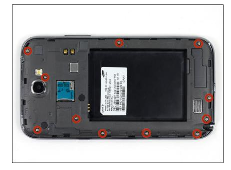
Remove the eleven 4.0 mm Phillips #00 screws securing the midframe to the display assembly.
