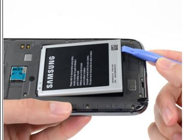
Insert a plastic opening tool, or your finger, into the notch of the battery compartment and lift the battery upward.
