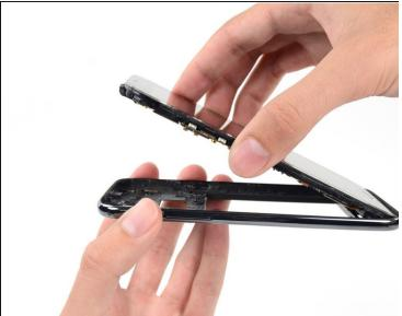
• Lift the display assembly out of the midframe.
