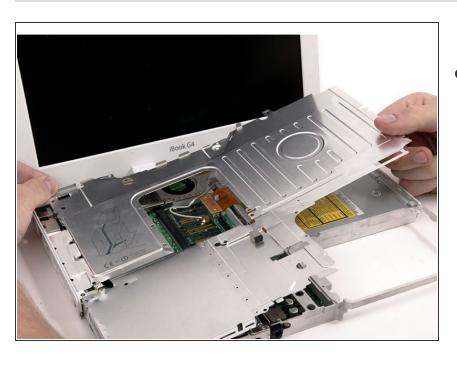
Lift the top shield up from the right side, minding the upper left corner, which may catch on the metal framework.
