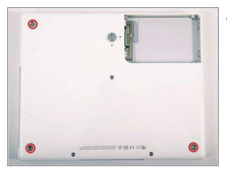
Remove the three newly-revealed Phillips screws.
