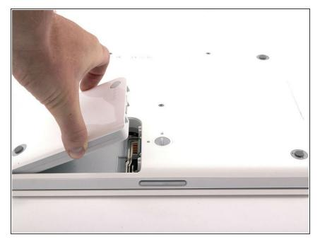
Lift the battery out of the computer.
