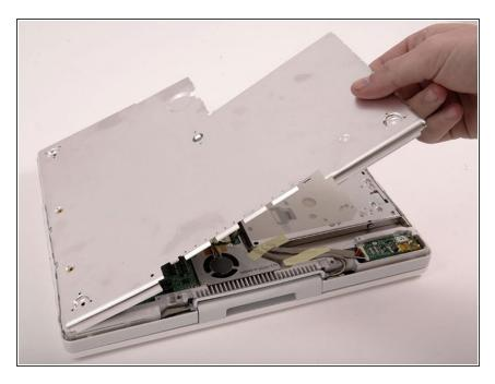
Lift the bottom shield off.
