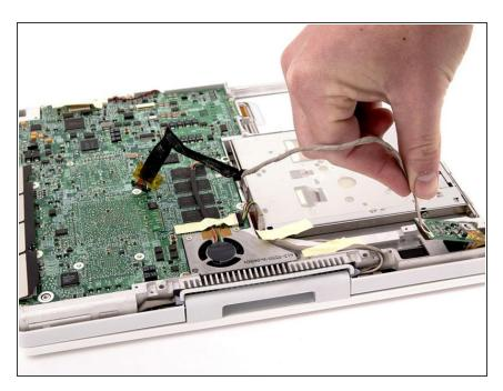
Deroute the cable from around the optical drive, removing tape as necessary, and angle the DC-In board out of its compartment.
