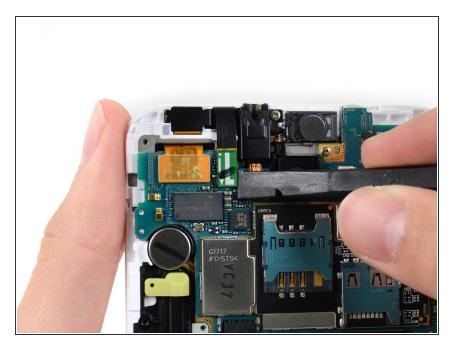
Use the flat end of a spudger to disconnect the headphone jack/earpiece speaker assembly cable connector.
