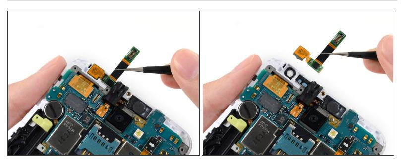
Using tweezers, or your fingers, remove the front-facing camera assembly.
