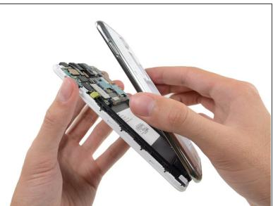
Remove the midframe from the display assembly.
