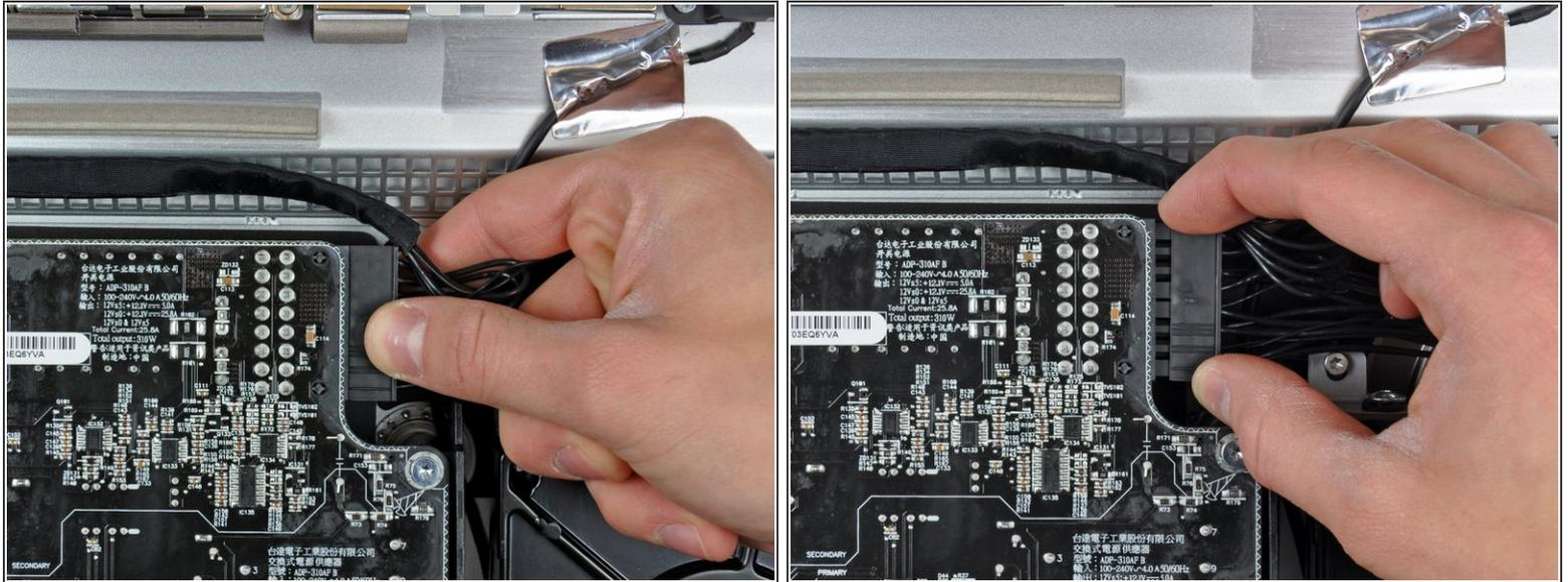
**⚠** The next few steps bring your hands close to the exposed face of the power supply. To avoid a high voltage shock from the many large capacitors attached to the board, **do not** touch the face of the power supply.
