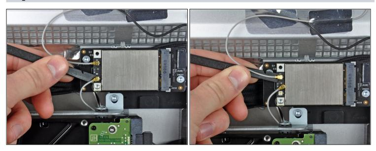
• Use the flat end of a spudger to pry both AirPort antenna cable connectors up off the AirPort card.
