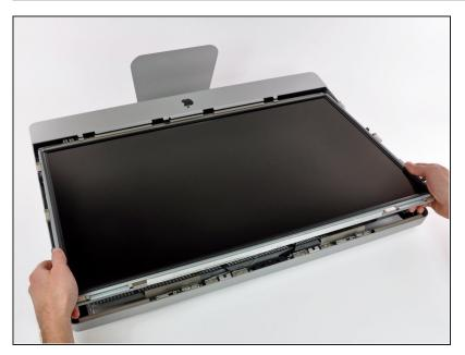
Carefully pull the display toward the top edge of your iMac and lift it out of the outer case.
