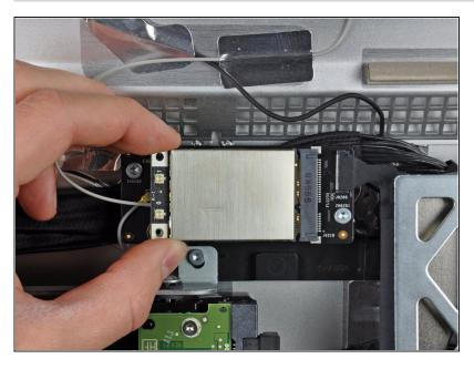
Pull the AirPort card away from its socket and remove it from the iMac.
