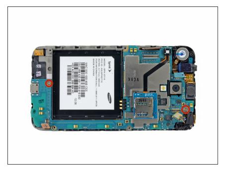
Remove the two 3 mm Phillips #00 screws.
