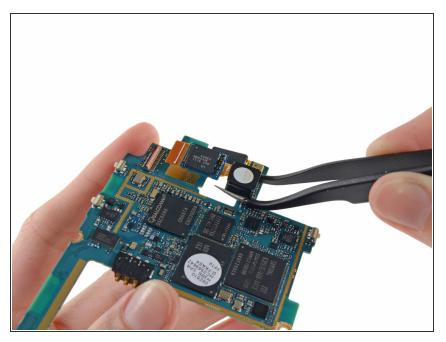
Remove the rear-facing camera from the motherboard.
