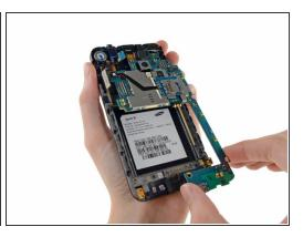
Lift the micro-USB end of the motherboard away from the display assembly and pull it down.
