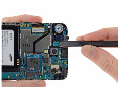
• Use the flat end of a spudger to disconnect the headphone jack/vibrator assembly cable.
