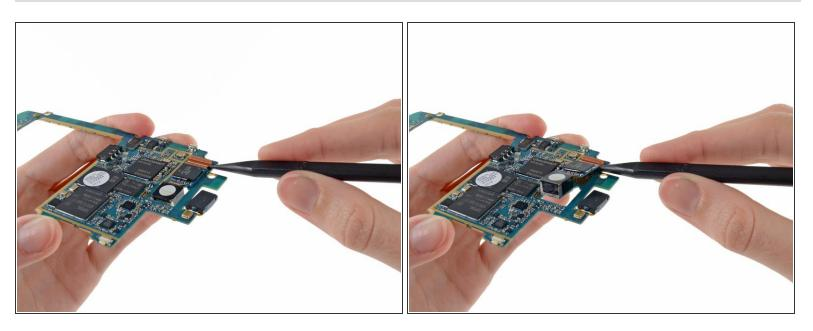
Slide a spudger under the rear-facing camera cable to free it from the adhesive.
