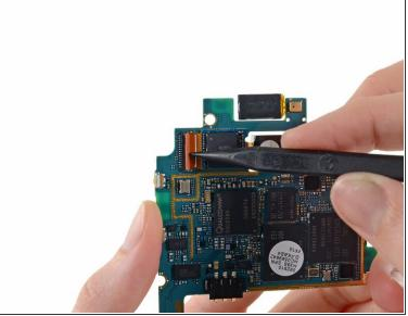
Use the pointed end of a spudger to flip the tab on the rear-facing camera ZIF connector.
