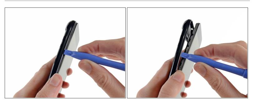
Pry again about two inches to the right of the volume control toggles between the midframe and the front panel assembly.
