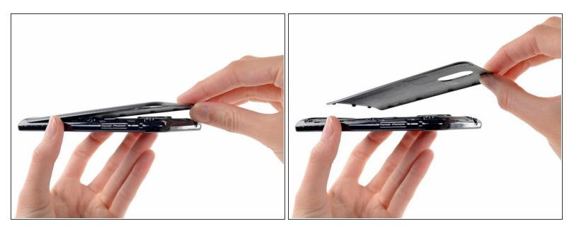
Lift and remove the rear case.
