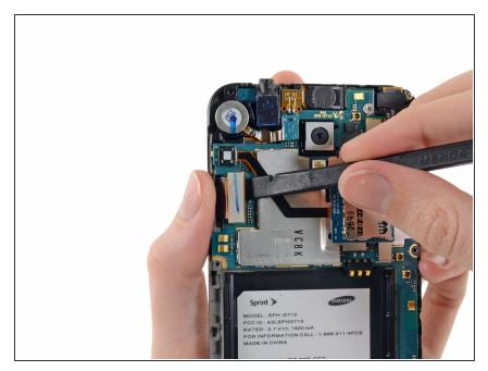
Use a spudger to disconnect the display cable connector.
