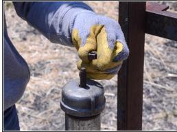
Loosen and remove both the pump rod jam nut and pump rod nut on the top of the slider.
