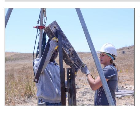
Remove the head and handle, and place them on a clean surface to prevent contamination.
