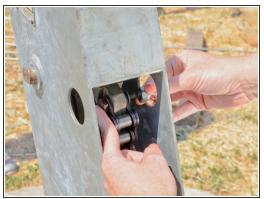
Remove the nut from the chain bolt.
