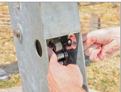
Remove the washer from the chain bolt.
