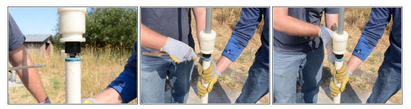
• Loosen the jam nut beneath the pump handle using the Tara tool.
