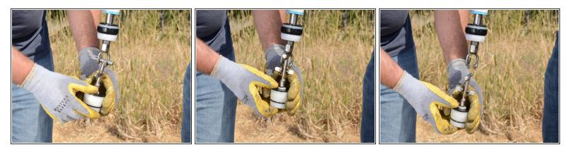
• Lift and twist the foot valve to unhook it from the traveling valve.
