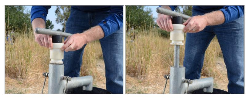
Pull the plastic bushing and handle straight up out of the pump.
