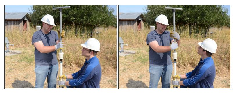
• Unscrew the pump handle from the top of the riser main.
