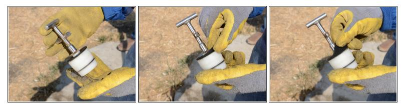
Inspect the foot valve for signs of wear or damage.
