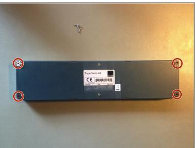
Remove the four bottom screws with a Phillips #00 screwdriver.
