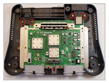
Remove the four screws indicated using the #1 Phillips screwdriver.
