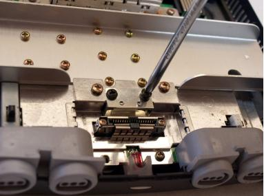
Remove the fourteen screws indicated in the example using the larger Phillips screwdriver.
