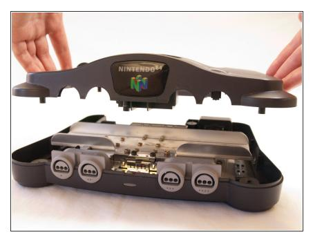
Rotate to top side up and lift off top cover.
