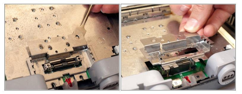
Remove the small metal bracket behind the expansion slot using the spudger.
