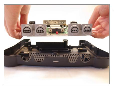
Lift up and remove the motherboard.
