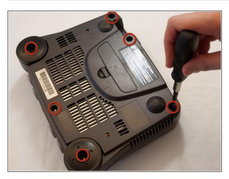
Remove the six screws on the bottom side indicated in the example with a gamebit head or screwdriver.
