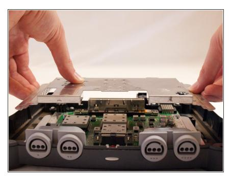
Lift off and remove the metal plate as indicated in the example.
