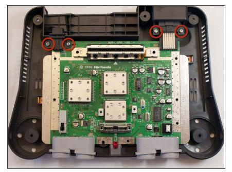
Remove the four screws indicated using the #1 Phillips screwdriver.
