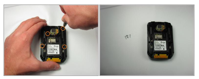
• Unscrew and remove all 4 T6 Torx screws.
