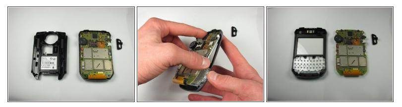
• Lift and remove inner back cover and set aside.
