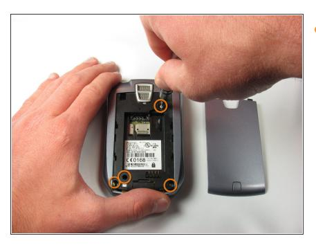
Unscrew and remove all four T6 Torx screws.
