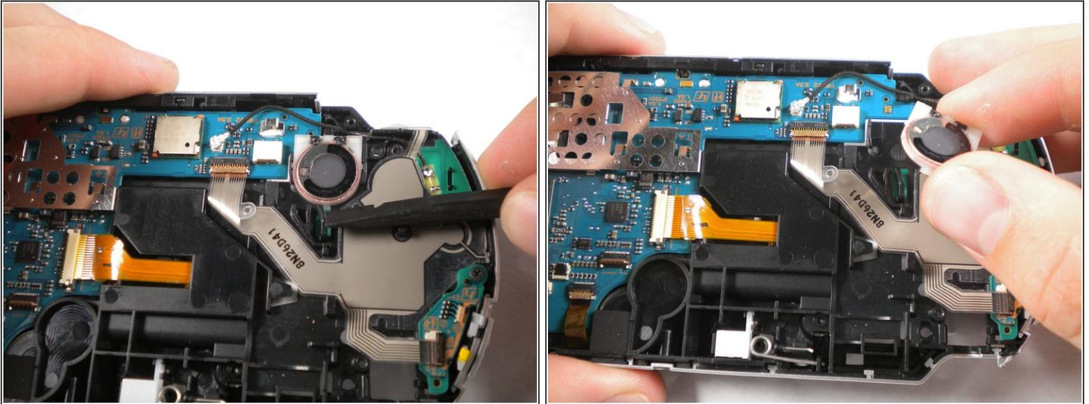
**⚠** Push the black tab at the bottom of the speaker to pop the speaker out of place, and remove the speaker.
