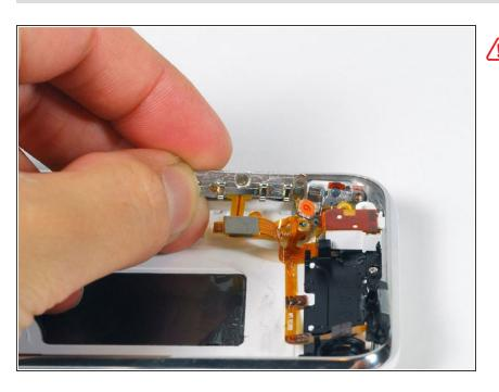
Lift the volume button circuitry away from the side of the iPhone, and carefully peel up the orange ribbon cable from the rear case. The cable is thin and easily damaged.
