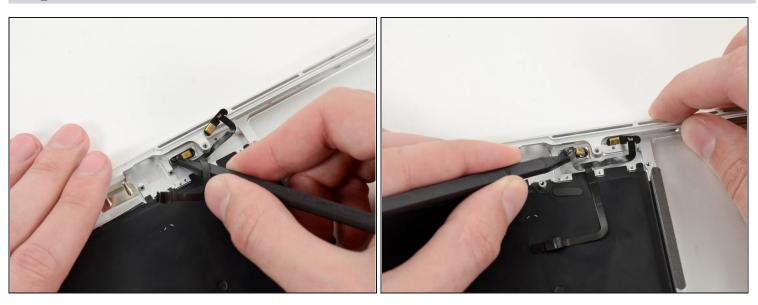
• Carefully pry the first microphone up off the upper case.
