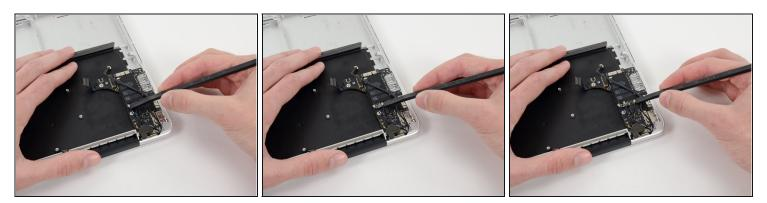
• Use the flat end of a spudger to pry and disconnect the three antenna cable connectors from the AirPort board.
