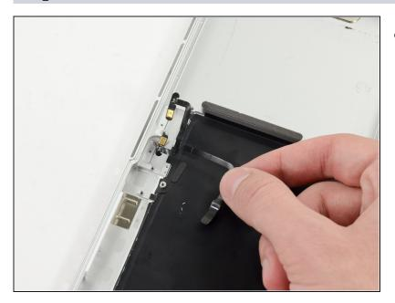
• Lift and remove the microphone assembly out of the upper case.
