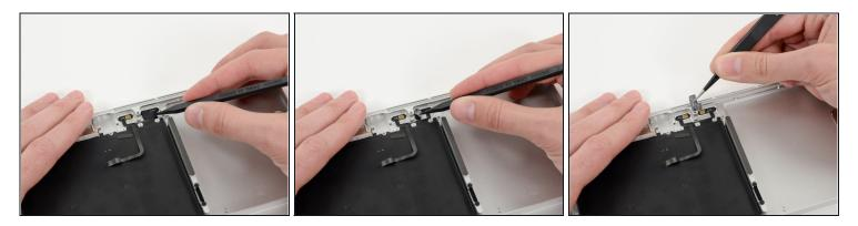
• Repeat the same procedure as the previous step to remove the tape covering the second microphone.
