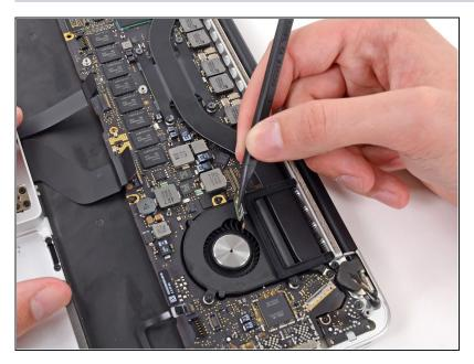
• Move the left fan ribbon cable aside to reveal a hidden screw securing the logic board assembly to the upper case.
