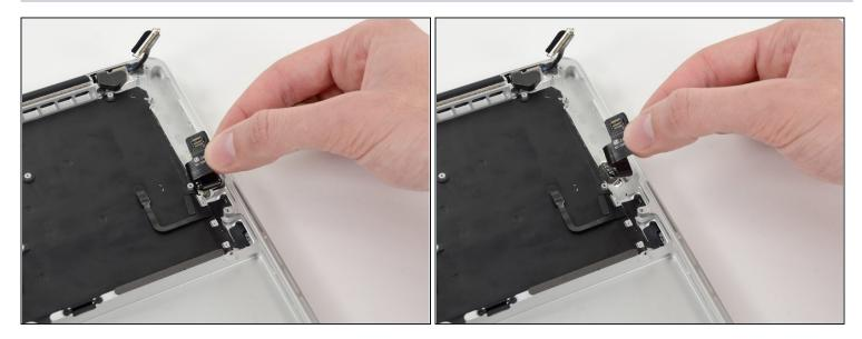
• Lift and remove the headphone jack out of the upper case.
