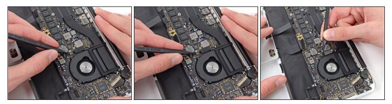
• Use the tip of a spudger to flip up the retaining flap on the left fan ribbon cable ZIF socket.
