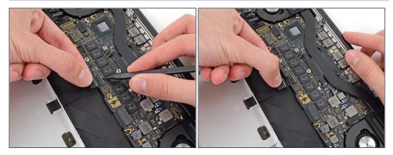
• Use the tip of a spudger to flip up the retaining flap on the trackpad ribbon cable ZIF socket.
