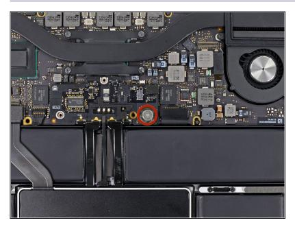
• Remove the wide head 6.4 mm T6 Torx screw securing the battery connector to the logic board assembly.
