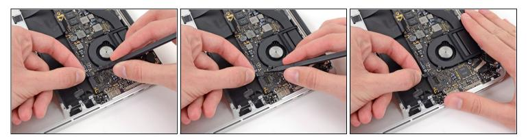
• Use the tip of a spudger to flip up the retaining flap on the microphone ribbon cable ZIF socket.
