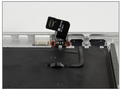
• Remove the two 3.4 mm T5 Torx screws securing the headphone jack to the upper case.
