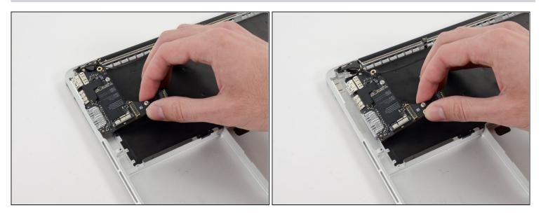
• Carefully pull and remove the I/O board away from its recess in the upper case.
