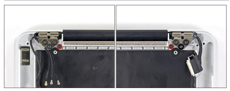
• Remove the 3.2 mm T5 Torx screws (one on each side) securing the aluminum hinge brackets to the upper case.
