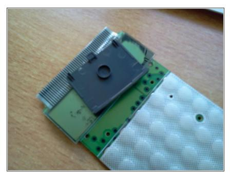
This must separate the front cover from the board. Remove the board and turn it over to view the front side with a soft black cushion cover over a smooth shinny mesh.
