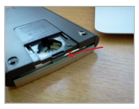
Use a flathead screwdriver to gently part the bottom and top cover at the hinge on the top.
