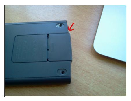
Remove the battery cover by sliding it out.
