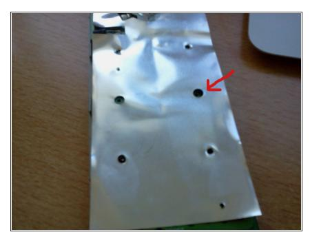
Removing the back cover to reveal the foil, unscrew the 4 screws holding the foil and 4 other holding the printed circuit board to the front cover.
