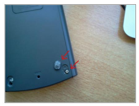
Firstly on the back cover, remove the small sticky soft cushioning material covering the recess with the screws in it. 4 of them in total. Unscrew them.
