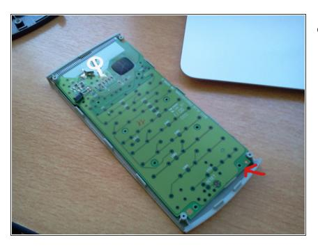
Remove the foil. Ensure all screws are off.
