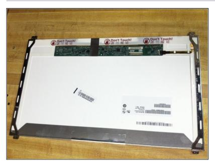
Finally, be sure that you order a new LCD that has the same backlight, resolution, and model number as the original.
