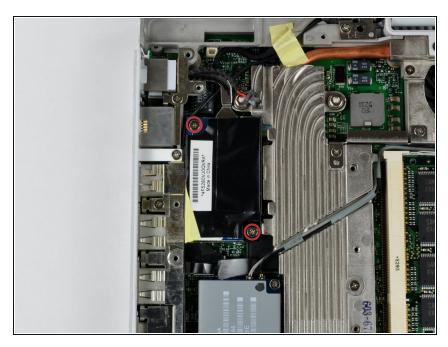
• Remove the two Phillips screws at the corners of the modem.
