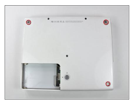
Remove the three newly-revealed Phillips screws.
