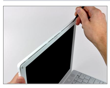
Run your spudger along the top edge of the front display bezel to evenly separate the two bezels.
