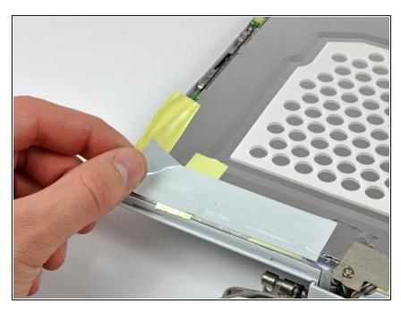
Remove the large piece of tape near the lower right corner of the display.
