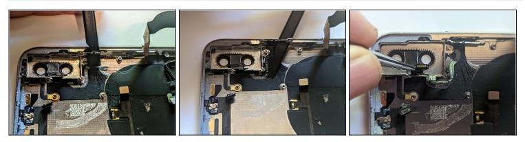
• Peel the flex cable from the frame.
