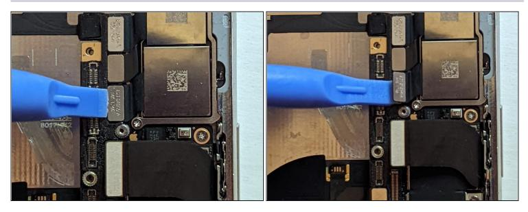
• Disconnect the Telephoto Camera cable connector.
