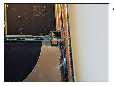
• When the SIM card is ejected, a pin slides out from the frame and pushes on the eject lever in the SIM card carrier. The pin needs to be pushed back into the frame so it will not block the removal of the logic board.
