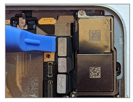
• Disconnect the Wide-Angle Camera cable connector.
