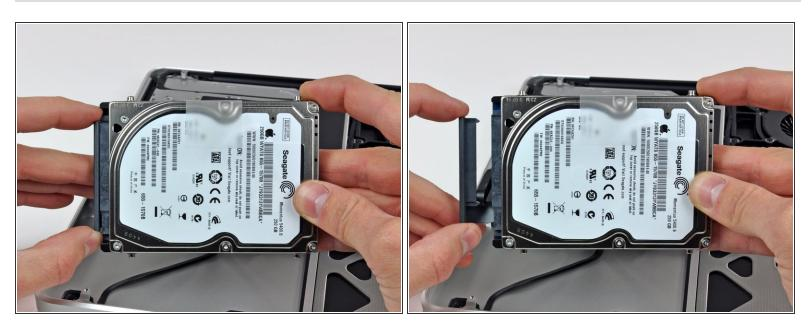
• Remove the hard drive cable by pulling its connector straight away from the hard drive.
