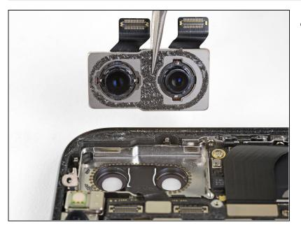
• Remove the rear-facing camera module.
