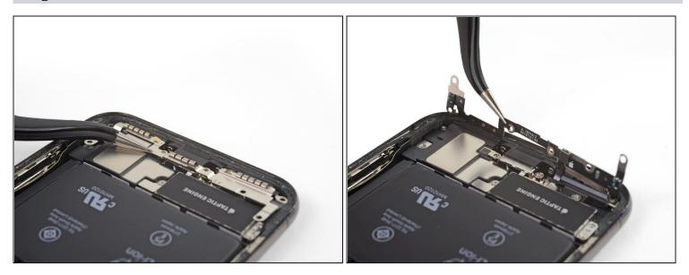
• Lift the bracket from the edge nearest the battery. Don't try to remove it fully, as it's still connected via a small flex cable.
