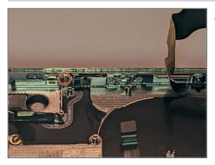
• Remove the remaining 2.0 mm Phillips screw securing the power button.
