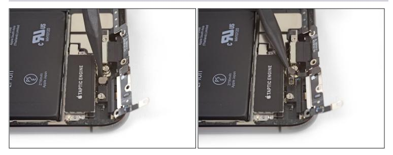
• While holding the bracket out of the way, use the point of a spudger to pry up and disconnect the flex cable underneath.
