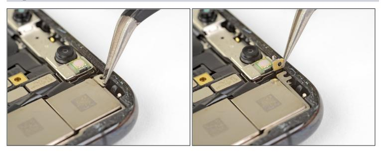
• Use <u>tweezers</u> to gently fold the small metal grounding bracket out of the way. Do not pull up on it as it is connected to a fragile flex cable.
