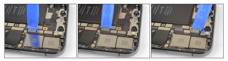
• Use an opening tool or fingernail to disconnect the two camera connectors by prying them straight up from their sockets.
