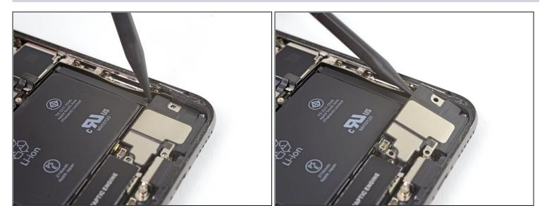
A When prying up the speaker, take care not to damage the flex cable you just disconnected. If necessary, hold it to one side so the speaker has room to come out.
