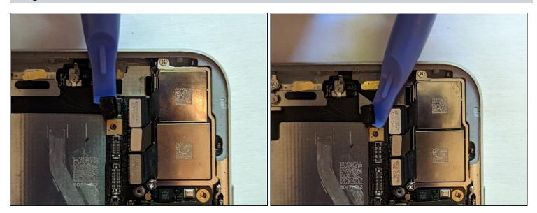
• Disconnect the WiFi Antenna cable connector.
