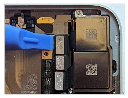
• Disconnect the Wide-Angle Camera cable connector.
