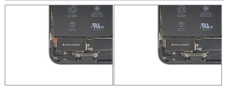
• Remove the 2.3 mm Phillips screw securing the Taptic Engine.
