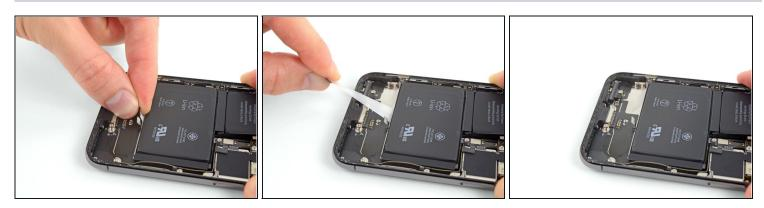
• Remove the center strip, being careful not to snag it on the speaker flex cable.
