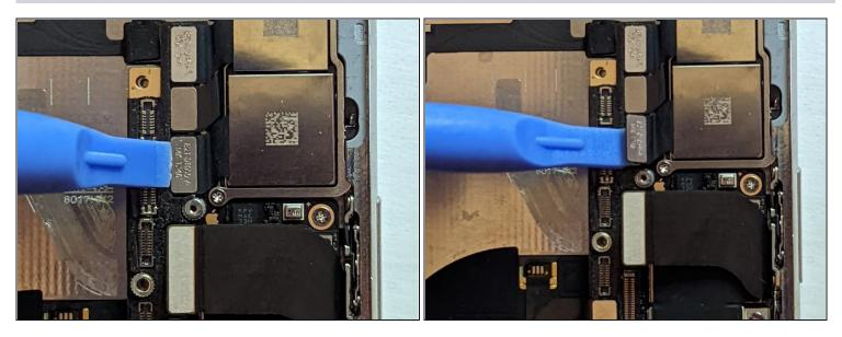
• Disconnect the Telephoto Camera cable connector.
