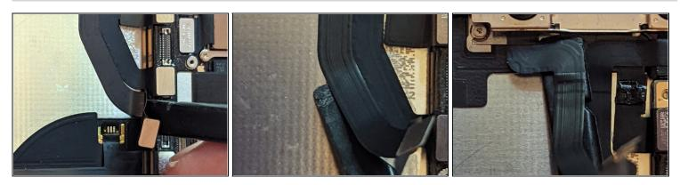
(i) The camera cables are lightly adhered to the midframe.
