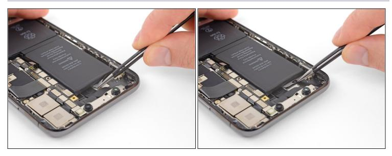
The final pull tab lies very close to the Face ID hardware. If damaged, Face ID can only be repaired by Apple, so work with care.
