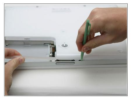
Run a spudger along the seam between the lower case and upper case on the front of the computer to free the tabs locking the lower case.
