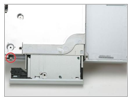
Pull the optical drive a bit more so that you can access and remove a second Phillips screw near the power receptacle.
