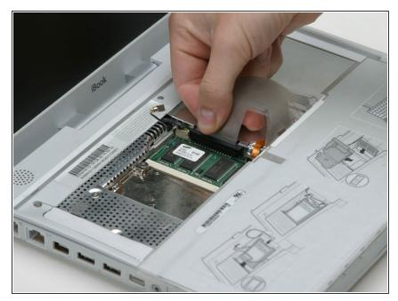
• Pull the keyboard cable up from the logic board, holding the cable as close to the connector as possible.
