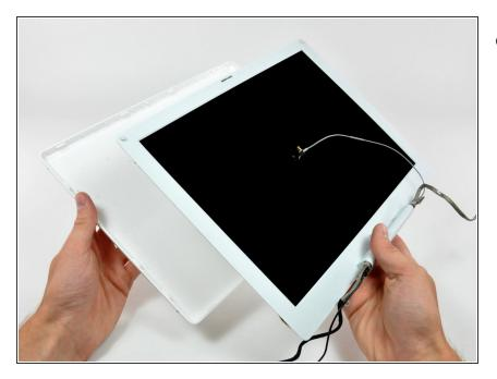
• Lift the rear bezel off the display.
