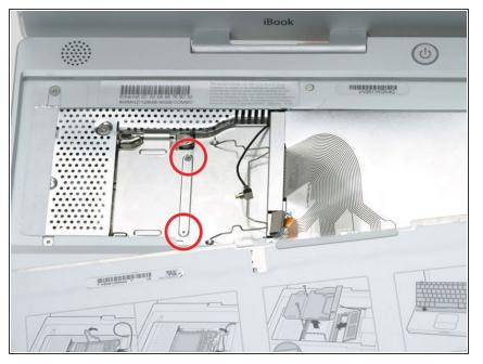
• Remove the two 2.5 mm Phillips screws that secure the RAM shield.
