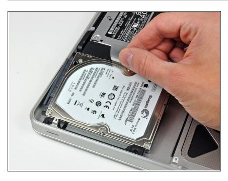
Lift the hard drive by its pull tab and pull it out of the chassis, minding the cable attaching it to the computer.
