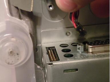
Remove the front panel connector. (You may also need to remove an additional screw that connects the front panel connector to the logic board assembly).
